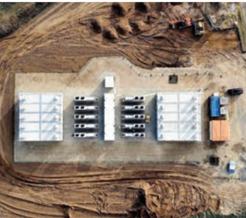
In Cremzow, a small municipality in northeast Germany where there is a heavy concentration of wind turbines, Leclanche has completed a **30.6 MW / 34.8 MWh** BESS to provide frequency regulation services. The Cremzow project, which was installed and commissioned in sections over a 6-month period, is jointly owned via an SPV by Enel Green Power (90%) and Enertrag (10%), the operator of the wind farm that surrounds the project site.
