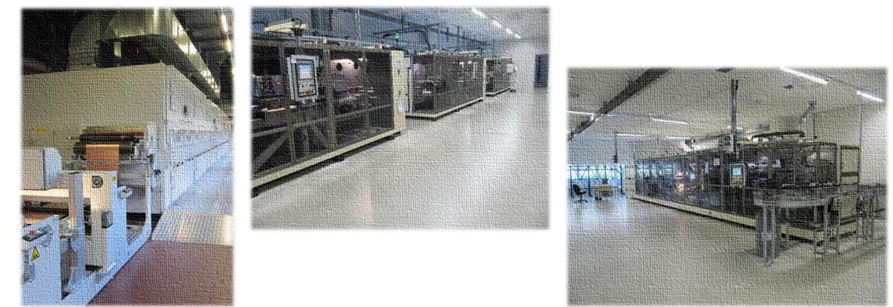
Fabrication steps: a part of coating line, electrode notching and cell assembly machines
